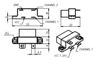
Device is equipped with four standard blade "FASTCON" terminals (6.3 mm x o.8mm). Five receptacles with insulation are supplied with the device, they are widely available in any electronics store.
